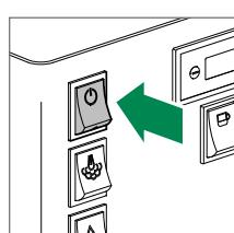
Shift the main switch to OFF to switch off the machine
