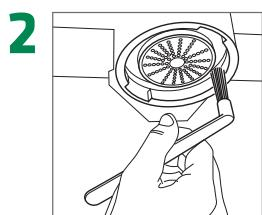
**2** Clean the portafilter gasket using the supplied brush
