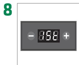
1St (1st Start Up): Wait for water loading to be completed in the coffee and steam boilers
