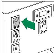
Move the main switch to OFF to switch off the machine
