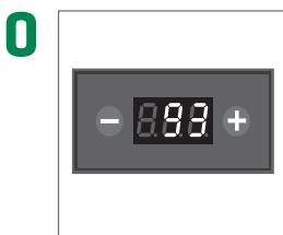
**10** At the end of the washing cycle the display will show the initial screen. Unlock the portafilter and remove the blind filter disk
