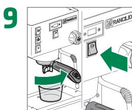
**9** Lock the portafilter back in place and press the coffee button to continue the washing cycle
