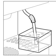
Submerge steam wand in water and heat it up
