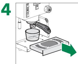
**4** Remove the grid and place a container to collect rinsing water
