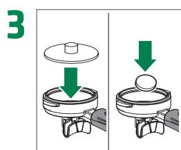
**3** Insert the blind filter disk and add the detergent supplied or an equivalent. Lock the portafilter
