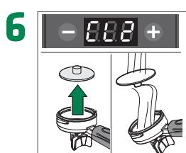
**6** When the display shows **CL2**, remove the portafilter with blind filter disk and rinse both with water
