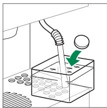
Submerge steam wand in milk cleaning solution
