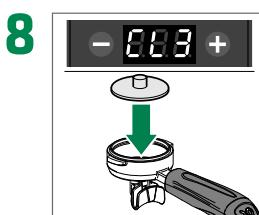
**8** When the display shows **CL3**, remove the portafilter and insert the blind filter disk once again
