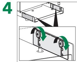
Secure the locking nuts and position the gliders
