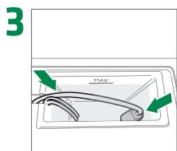
Ensure that the tubes are inserted in the reservoir and that the vacuum trap is fitted in the dedicated space inside the reservoir
