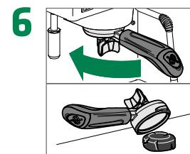
Remove the portafilter to empty and clean it, then lock it back in place
