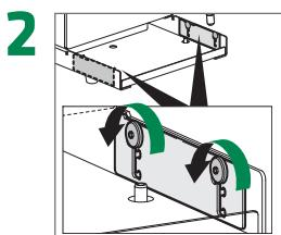
Loosen the locking nuts
