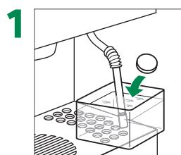
Submerge steam wand in milk cleaning solution
