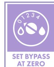
*The bypass on the iX Head when attached to the iX Vend filter, must be set to 0 to ensure no hard water is dialled back into the water supply.*
